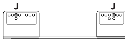
Drawer runner bracket screw position
