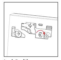
**Lock Position**Tighten screw shown to lock in position.
