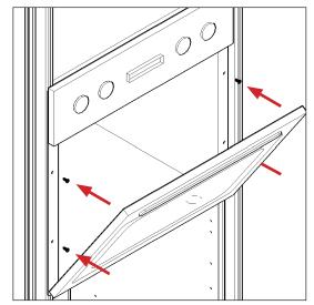
**Step3.** Re-insert the appliance and secure to the unit with screws.
